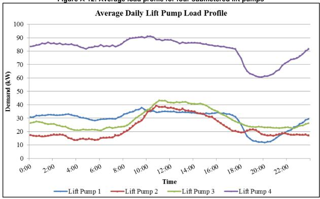
Figure A-13: Load curves for four submetered lift pumps
