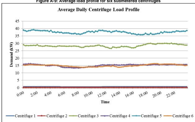
Figure A-9: Average load profile for six submetered centrifuges
