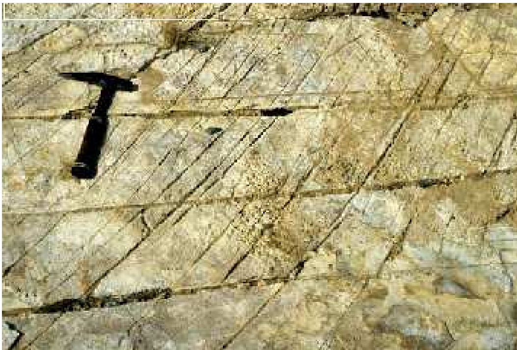
Figure 2. Field example of a fracture network composed of two or more sets of intersecting fractures having a dihedral ( i.e. , oblique, or non-orthogonal) intersection angle between the fracture planes.
