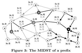
Fig. 3 shows the resulting MIDST for the prefix in the same example of Fig. 2. Anchors u, r, and o send their join requests towards d to join the MIDST of the prefix. The links that constitute the MIDST are indicated by solid lines in the figure, and multipoint data traffic for the prefix can flow in both directions of those links.
