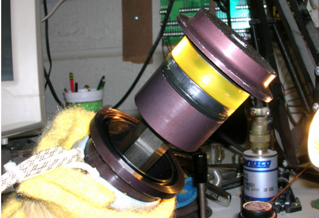
Figure 62. Resin injector with piston extended and resin 'puck' attached to end-plug
