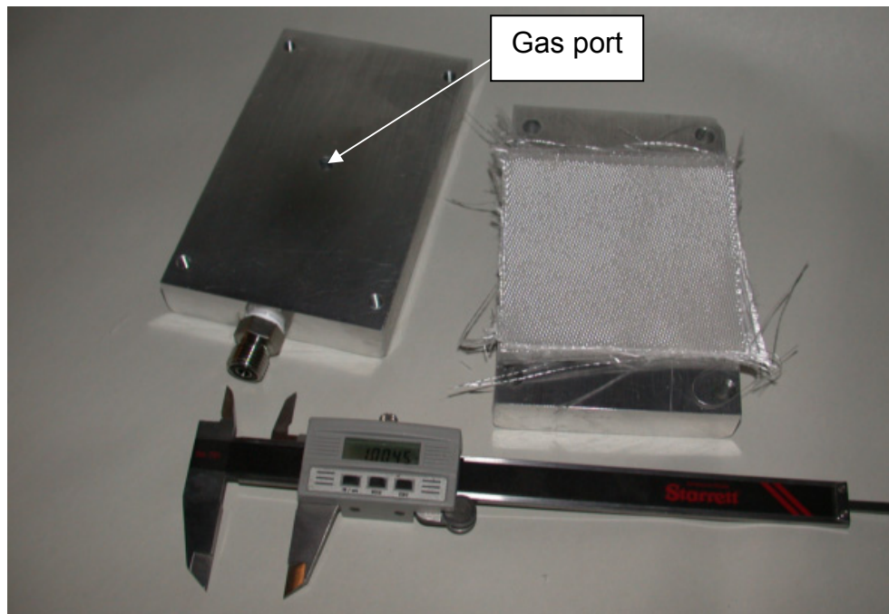
Figure 34. Glass preform sample for preform degassing tests
