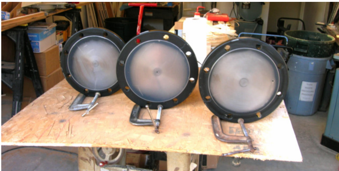
Figure 68. Mold plates during cleaning, seasoning and release agent application
