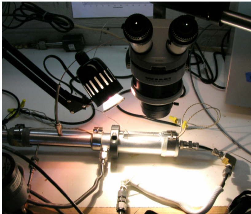
Figure 110. Setup for resin gas dissolution studies, thermal insulation not installed, microscope in position
