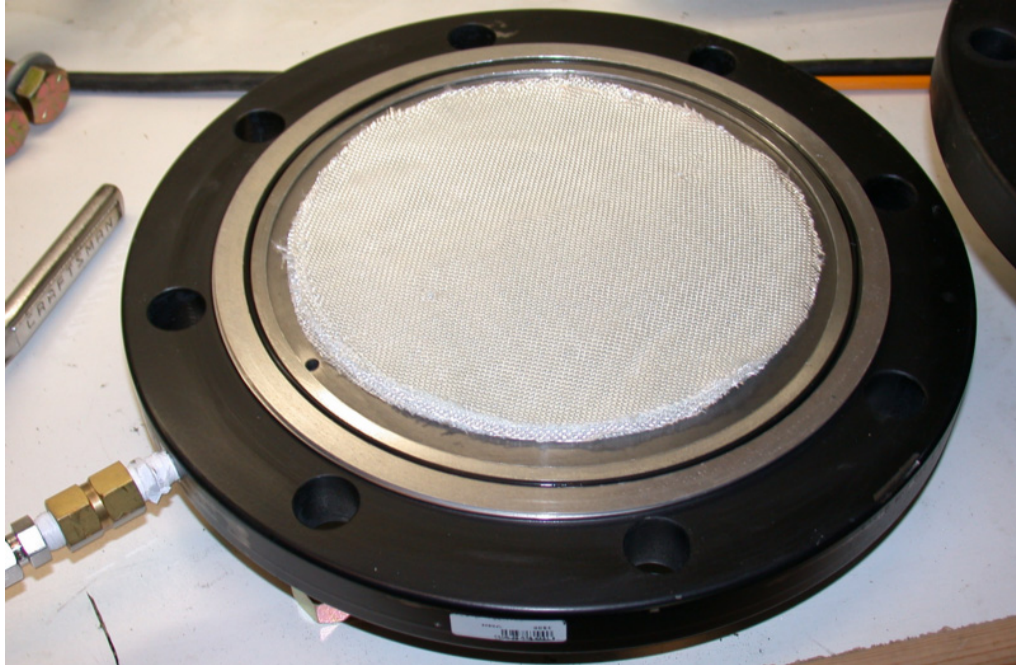
Figure 73. Glass preform, 10 plies ready for injection
