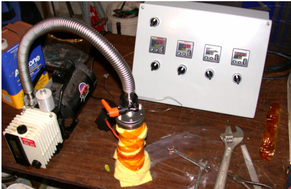
Figure 22. Vacuum chamber used to dry preform samples
