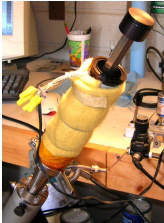
Figure 89. Resin injector with piston extended for cleaning
