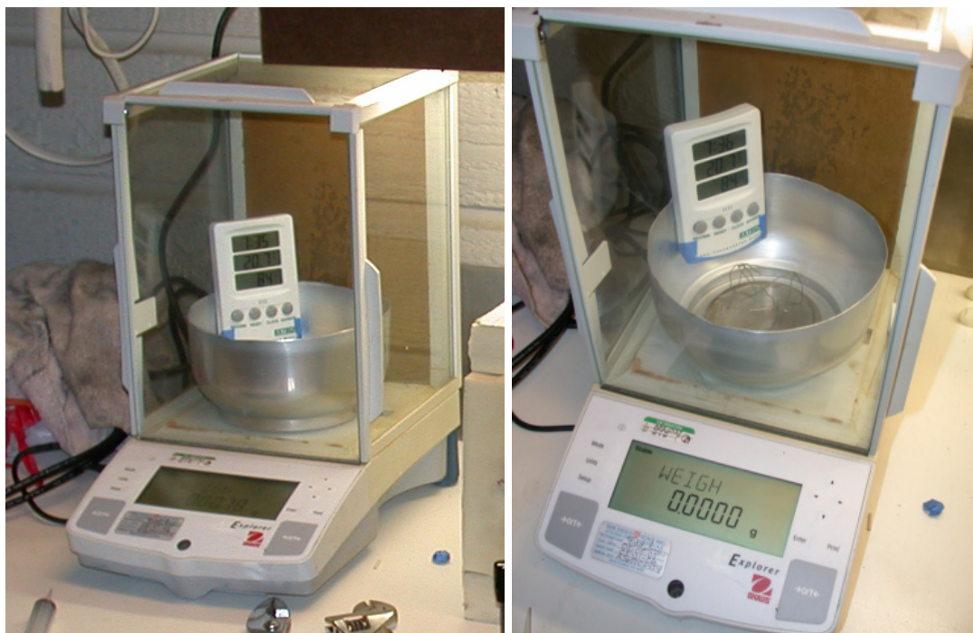
Figure 98. Microgram scale used to weight mass changes in preform samples
