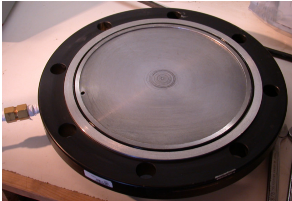
Figure 101. Panel mold bottom with aluminum rings and O-ring in position
