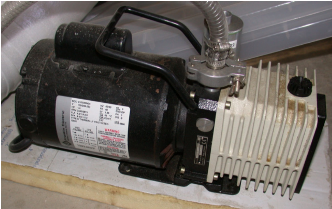
Figure 88. Varian vacuum pump used for all experiments
