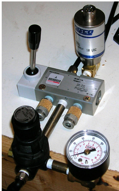
Figure 91. Pressure regulator, 3-way 5-port control valve and pressure transducer for resin injector control
