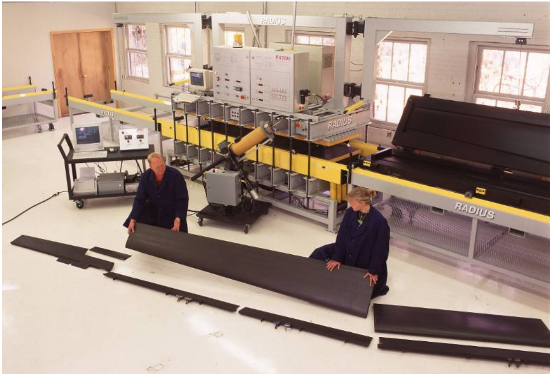
Figure 2. Aircraft control surfaces fabricated using resin transfer molding (source: Radius Engineering, Inc.)
