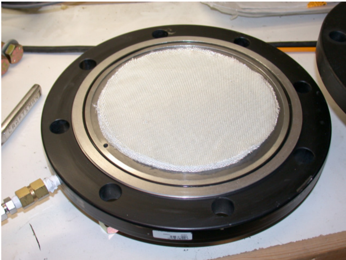
Figure 114. Glass fiber cloth positioned in panel mold
