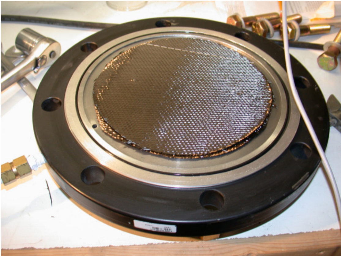
Figure 115. Stack of carbon fiber fabric positioned in panel mold
