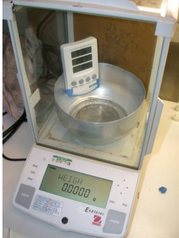
Figure 25. Precision scale used to measure fabric mass changes
