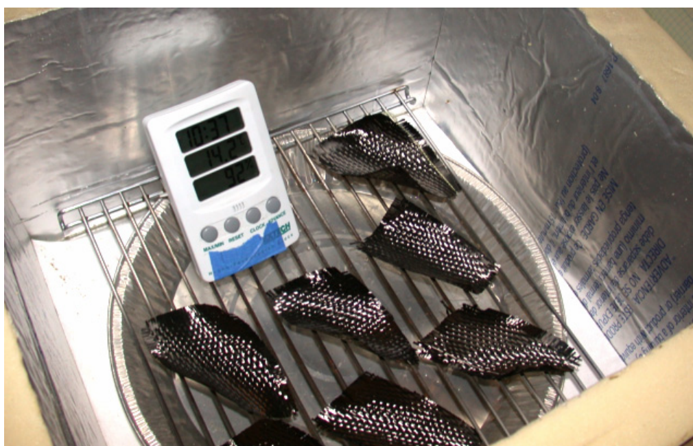
Figure 24. Carbon preform samples during aging in humidifying chamber
