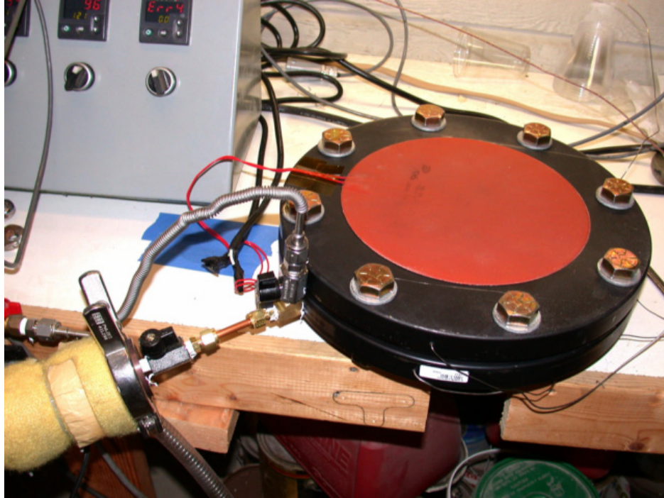
Figure 102. Panel mold closed and connected to injector. Note control TC inserted into flanges (foreground). Note red pad heater.
