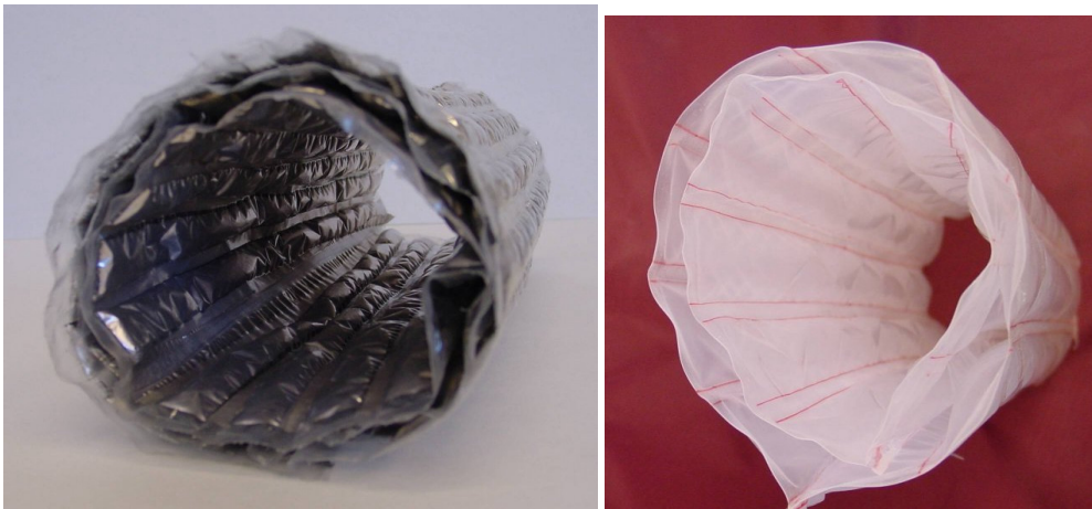
Figure 3. End view of longitudinal GFP duct sections: metallized on the left and non-metallized on the right. (Photo: Goudey, LBNL)
