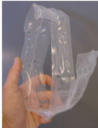
Figure 5. Helical construction for GFP duct sample. (Photo: Goudey, LBNL)
