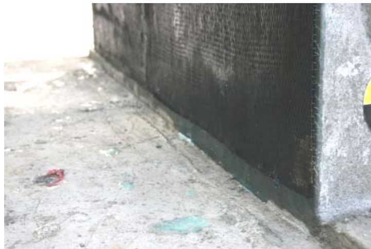
Figure 4.28: Test 6- CMU 3 CFRP at footing lip
