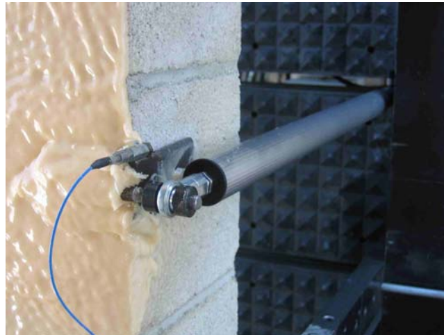
Figure 6.17: Connection of accelerometer and linear potentiometer, Tests 6 and 7
