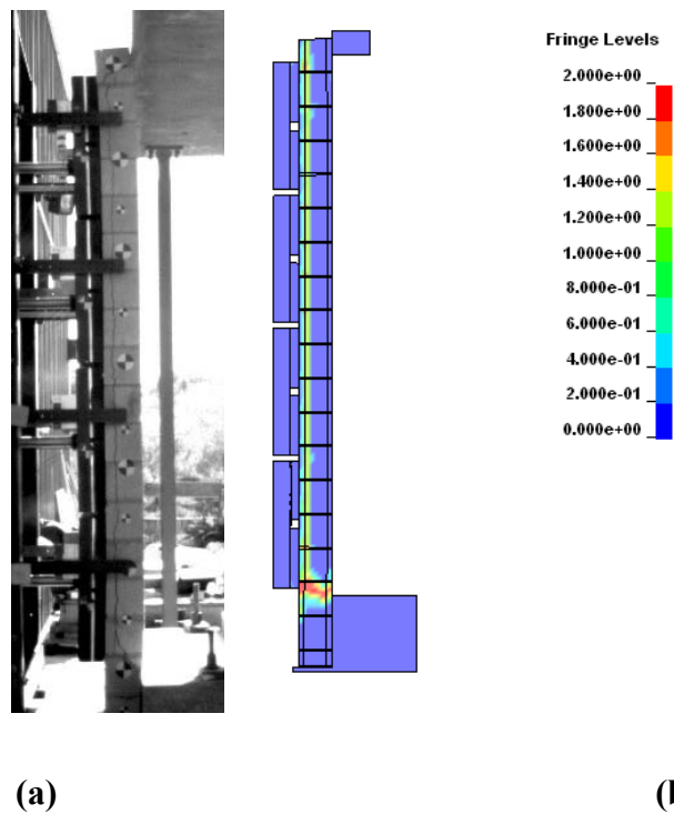
Figure 6.52: Damage for Test 2 after impact (a) Experiment; (b) FEA
