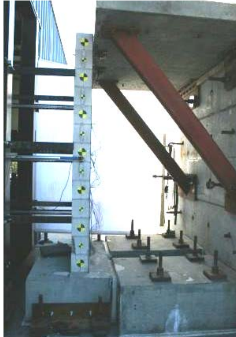
Figure 4.13: Test 1- CMU 1 post test
