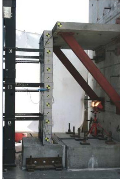
Figure 4.30: Test 6- CMU 3 post test
