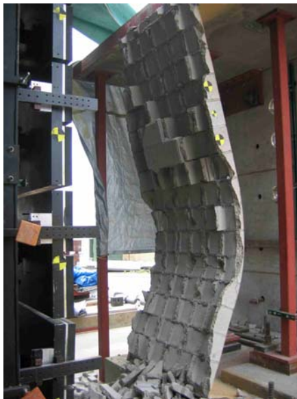
Figure 6.43: Test 7 peeling overlap at bottom support
