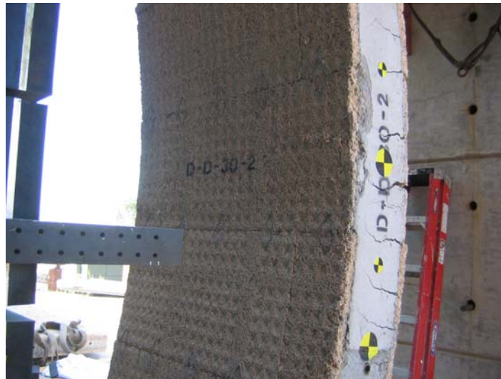
Figure 5.63: Permanent indentations in frangible panel
