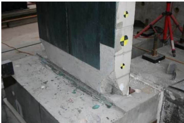
Figure 4.25: Test 6- CMU 3 removal of CFRP and concrete spall
