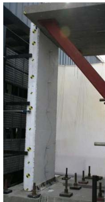
Figure 5.37: Specimen accelerometer locations
