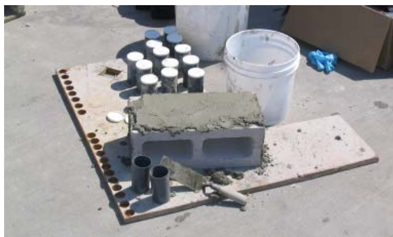
Figure 3.29: Grout material test specimens
