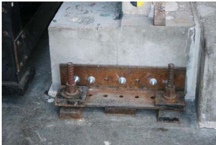
Figure 4.4: Connection of footing to reaction slab
