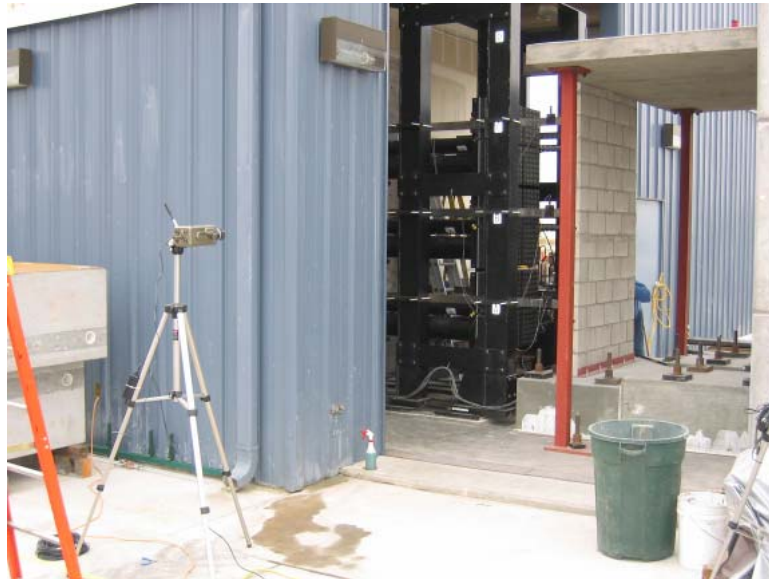
Figure 3.27: Location of phantom camera for 6 in. thick CMU wall tests
