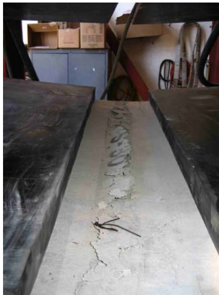
Figure 5.15: Series I Static Test 5- RC-S-30 concrete crushes
