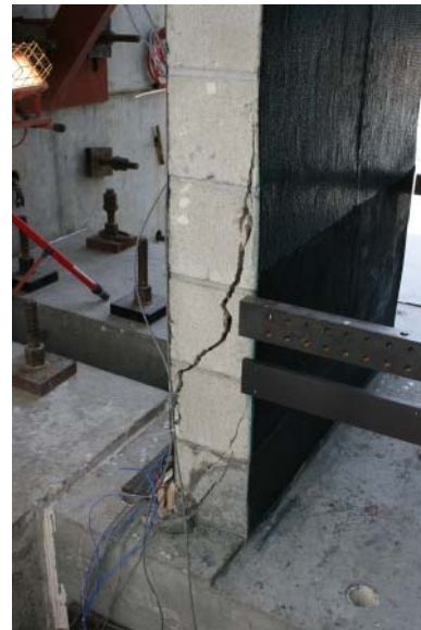
Figure 4.30: Test 6- CMU 3 post test
