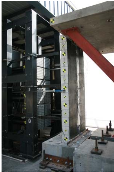
Figure 4.20: Test 4- CMU 2 post test
