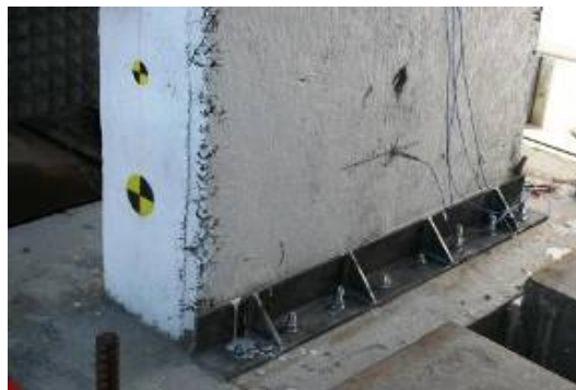
Figure 5.43: Series II angle detail
