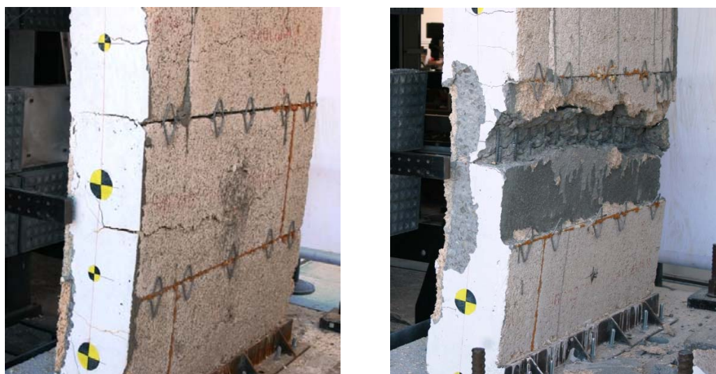
Figure 5.50: RC-8-3 (lap splice) post single BG impact
