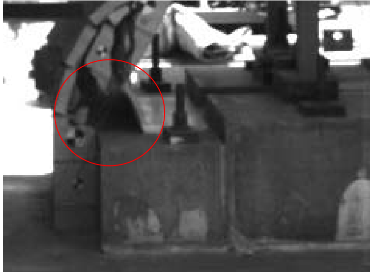
Figure 6.43: Test 7 peeling overlap at bottom support
