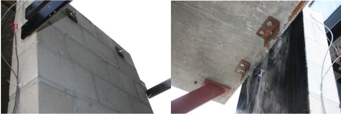
Figure 4.5: Tie back connection at top
