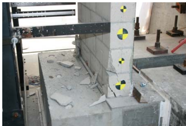
Figure 4.21: Test 4- CMU 2 damage at bottom
