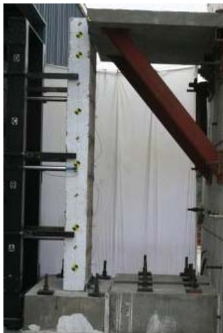
Figure 5.35: Tracking targets on specimen
