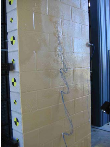
Figure 6.20: Strain gage wires
