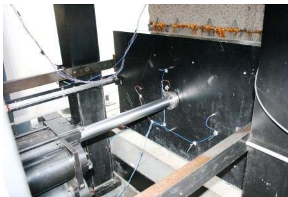
Figure 4.8: BG accelerometers configuration
