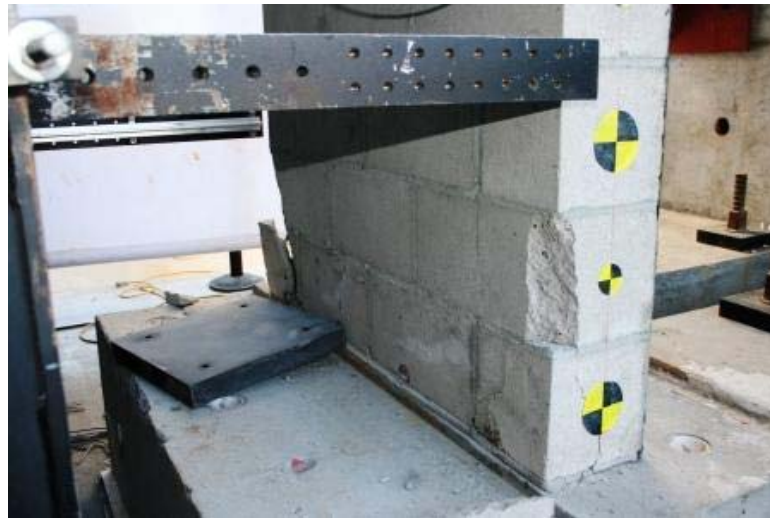
Figure 4.14: Test 1- CMU 1 bottom support post test
