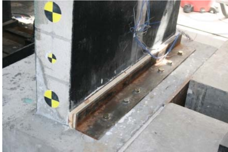
Figure 4.29: Test 6- CMU 3 angle at base
