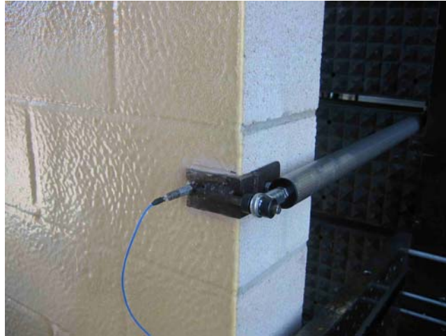
Figure 6.16: Connection of accelerometer and linear potentiometer, Tests 3-5
