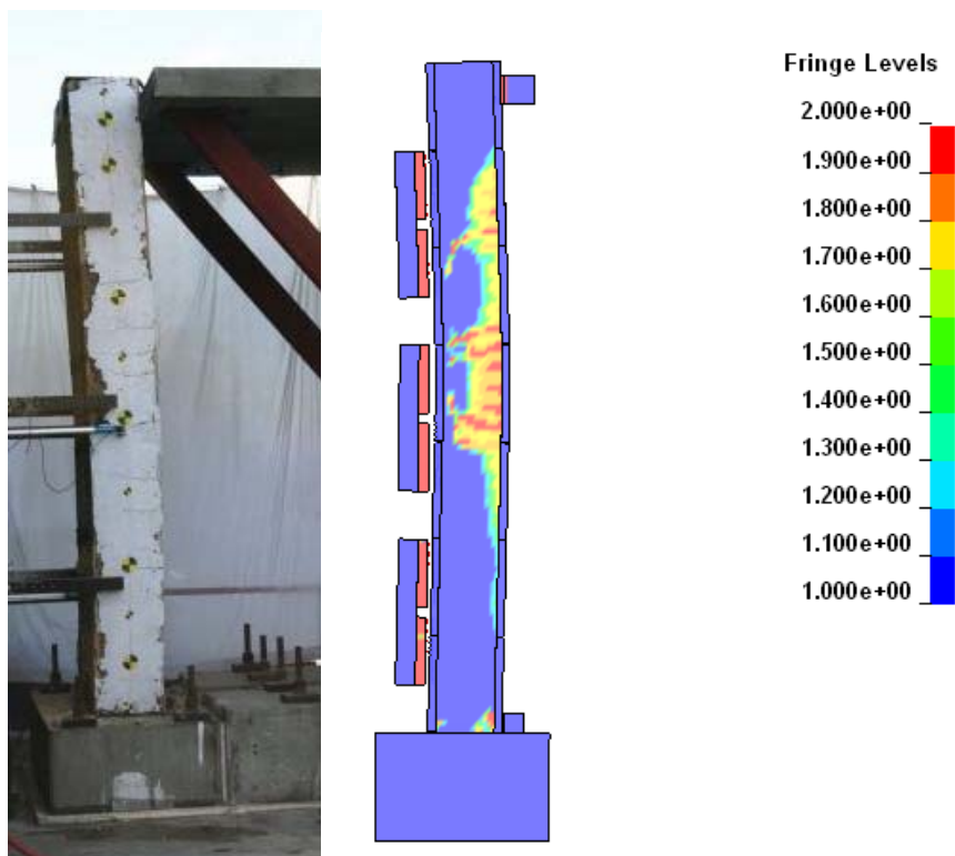
Figure 5.93: Comparison of damaged state for Series II
