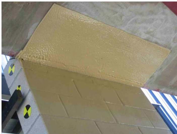
Figure 6.5: Top polyurea connection with 18 in. overlap
