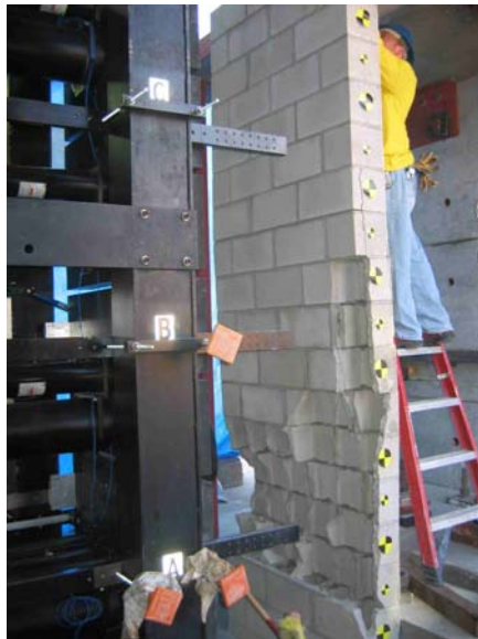
Figure 6.33: Test 4 front face post test
