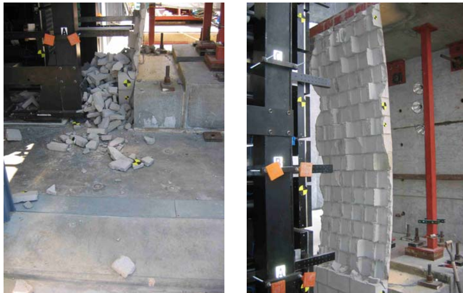
Figure 6.39: Test 6 peeling at bottom support after impact
