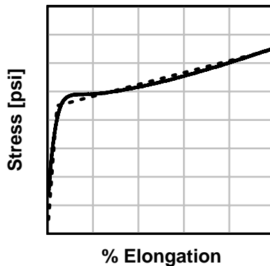
Figure 6.71: Constitutive relation of polyurea in uniaxial tension
