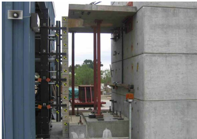
Figure 6.14: Test setup for URM walls
