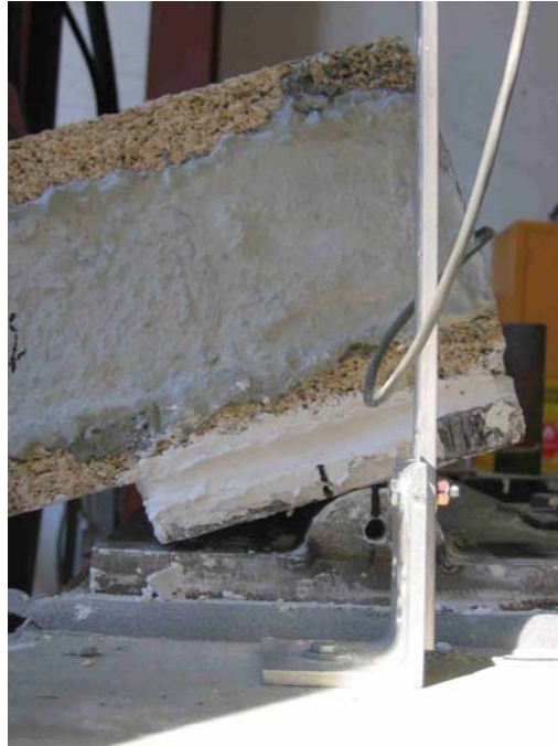
Figure 5.16: Static Test 7- FP-D-20-2 Support at 16 in. of displacement
