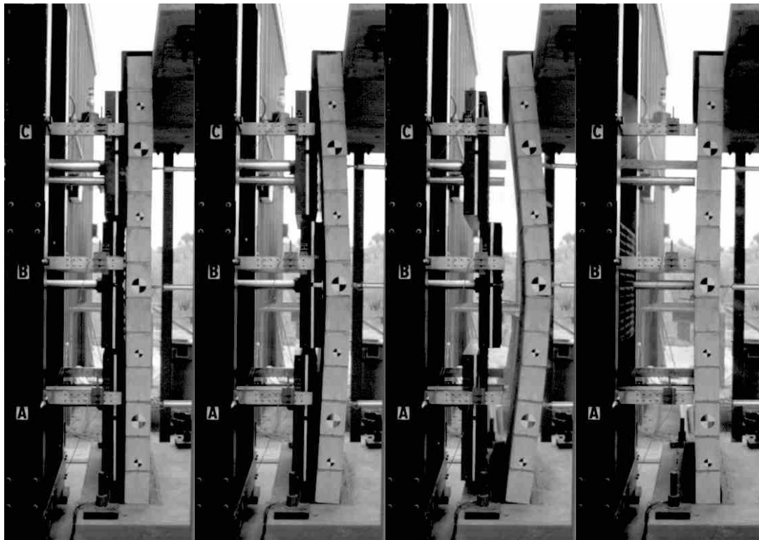
Figure 3.35: Photo sequence from 6 in. CMU Wall Test 1
