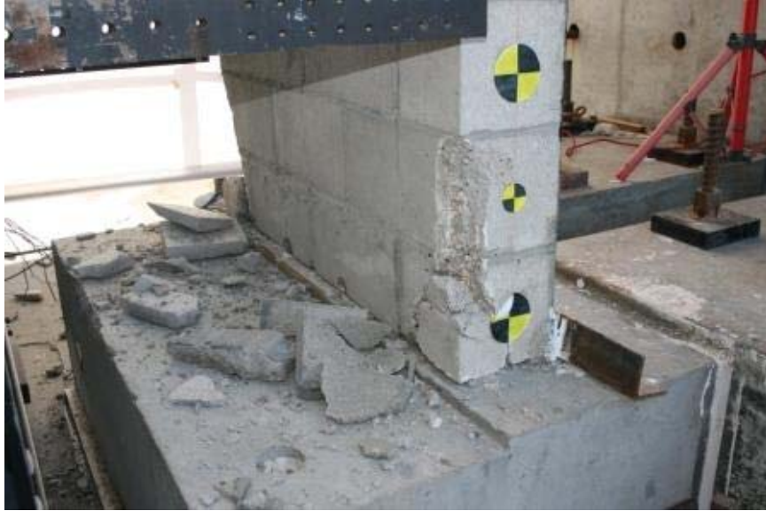
Figure 4.19: Test 3- CMU 1 bottom post test
