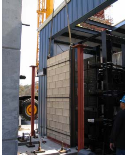
Figure 3.23: Placement of wall in test setup
