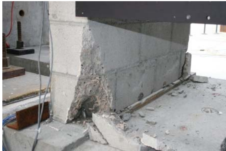
Figure 4.16: Test 2- CMU 1 bottom support post test
