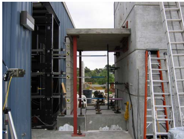
Figure 3.24: Setup for 6 in. thick CMU wall tests
