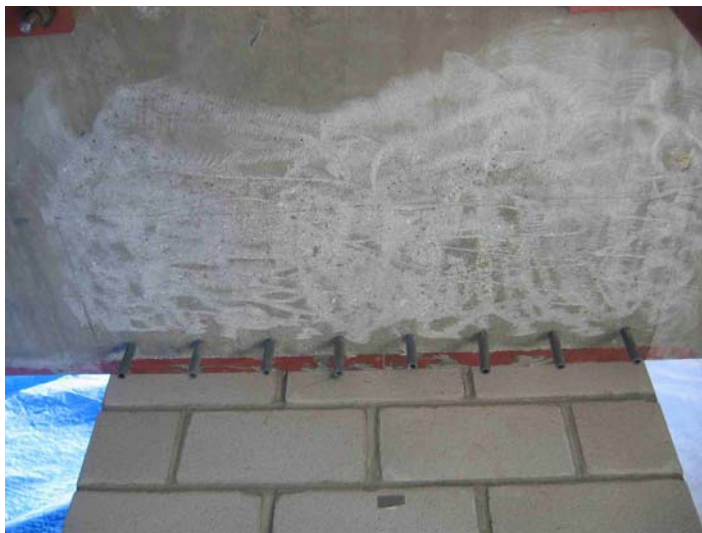
Figure 6.6: Wedge anchors at bottom support
