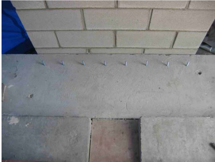
Figure 6.6: Wedge anchors at bottom support
