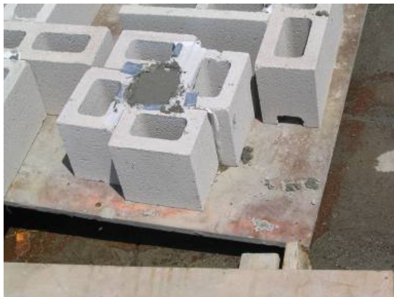
Figure 3.29: Grout material test specimens
