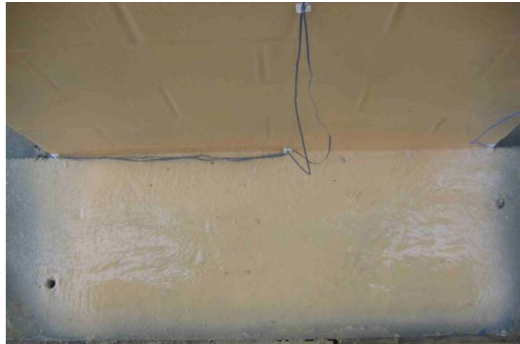
Figure 6.13: Bottom connection for polyurea with primer
