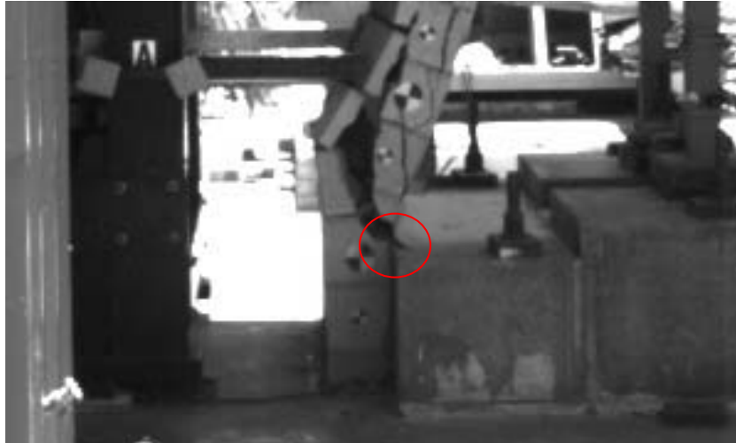
Figure 6.39: Test 6 peeling at bottom support after impact
