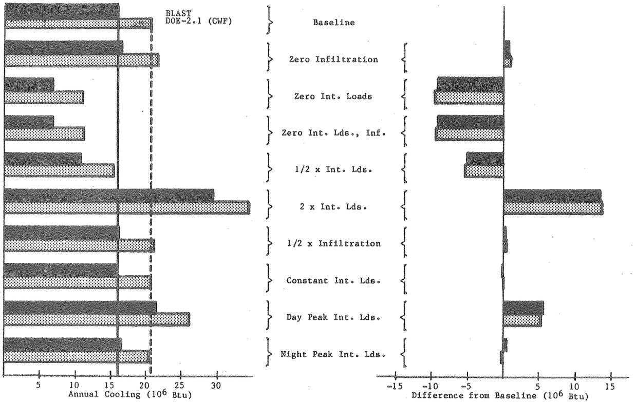
Figure 4.3b Effect of changes in internal loads and infiltration on annual cooling loads (Washington, D. C.)
