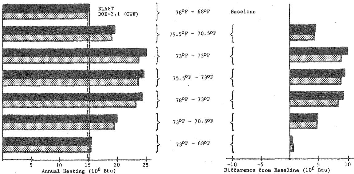
Figure 4.4a Effect of interior temperature setting on annual heating loads (Washington, D. C.).
