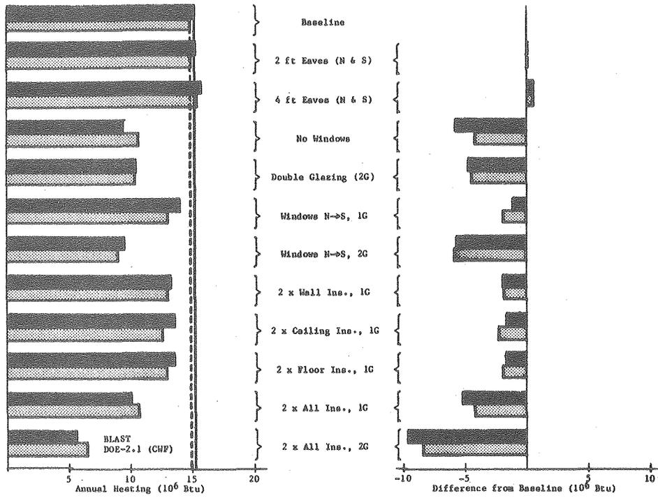
Figure 4.6a Effect of selected design changes on annual heating loads (Washington, D. C.)
