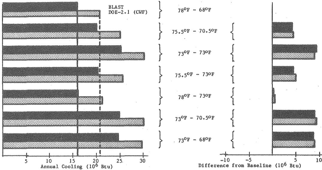
Figure 4.4b Effect of interior temperature setting on annual cooling loads (Washington, D. C.)
