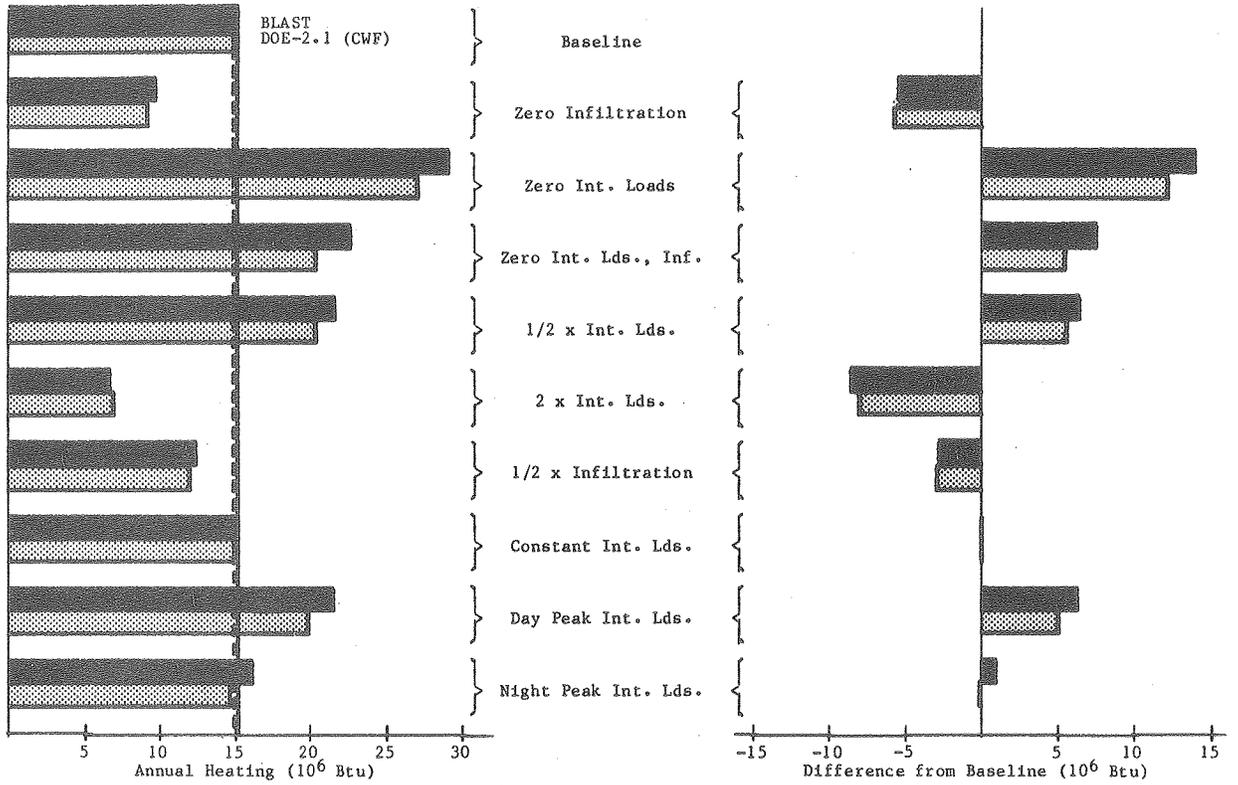
Figure 4.3a Effect of changes in internal loads and infiltration on annual heating loads (Washington, D. C.)
