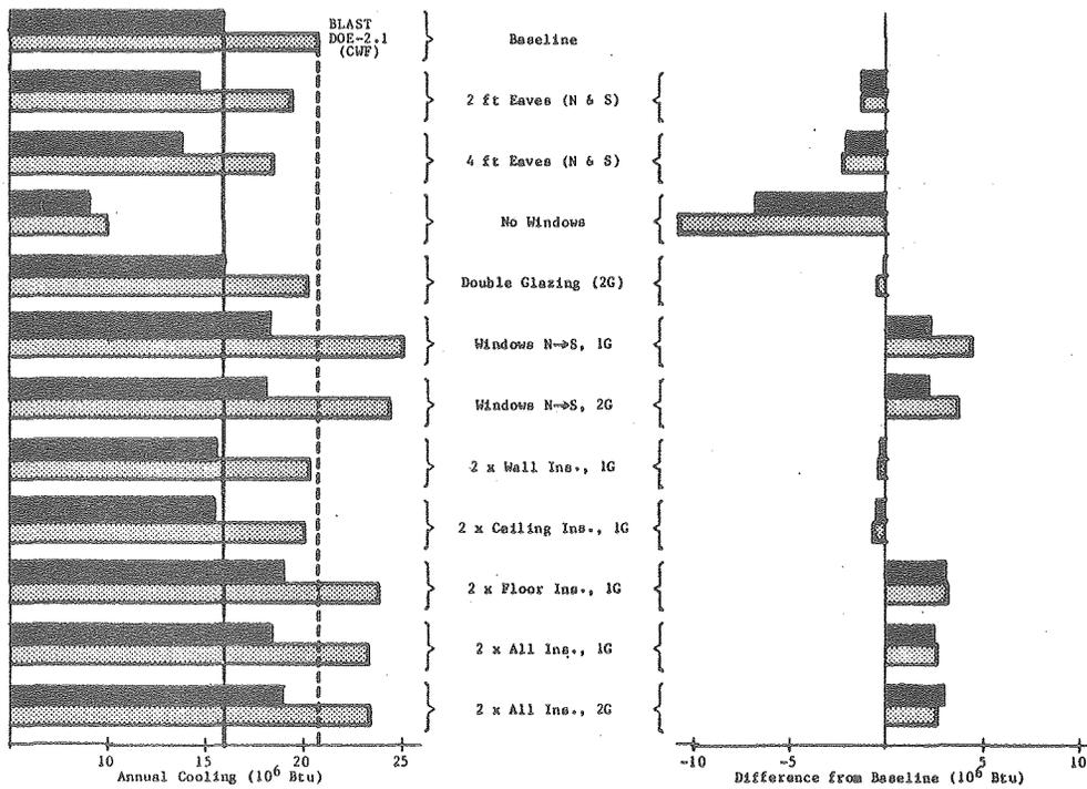
Figure 4.6b Effect of selected design changes on annual cooling loads (Washington, D. C.)
