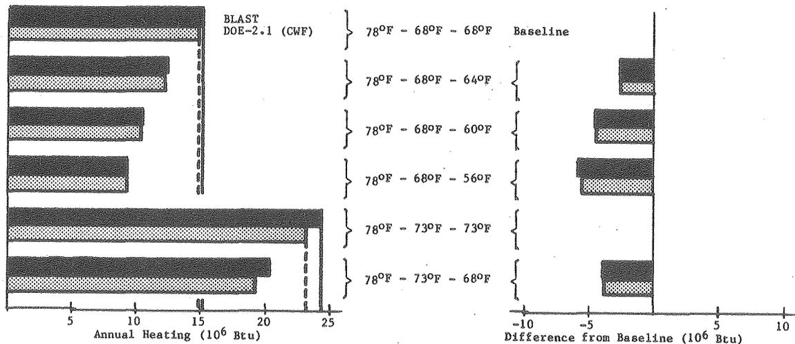
Figure 4.5a Effect of night setback on annual heating loads (Washington, D. C.)
