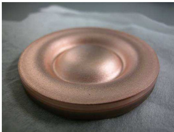
Figure 2.5: Copper sputter target with race track
