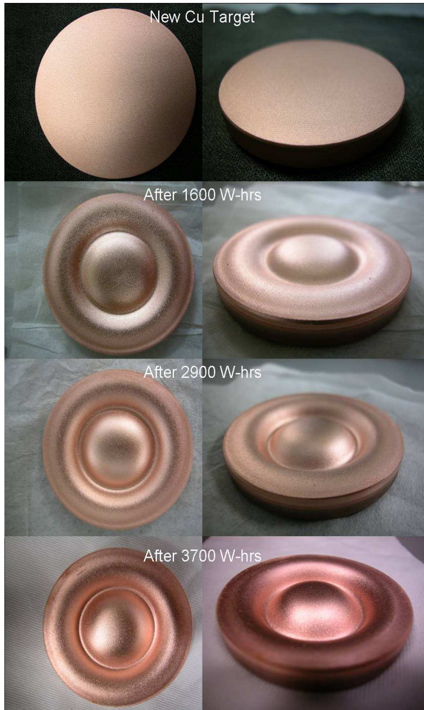
Figure 8.8: Comparison of the copper sputter target for different lengths of coating time
