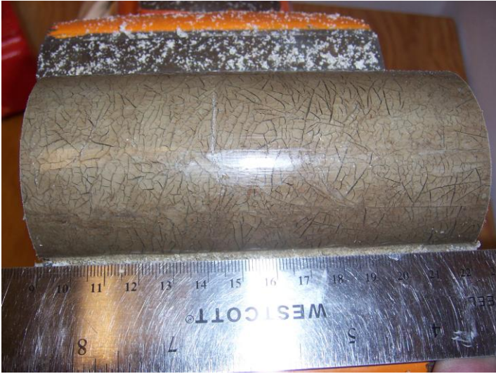
Figure 8. Cracks present throughout the clay-rich sample frozen in a pressure vessel in a freezer.
