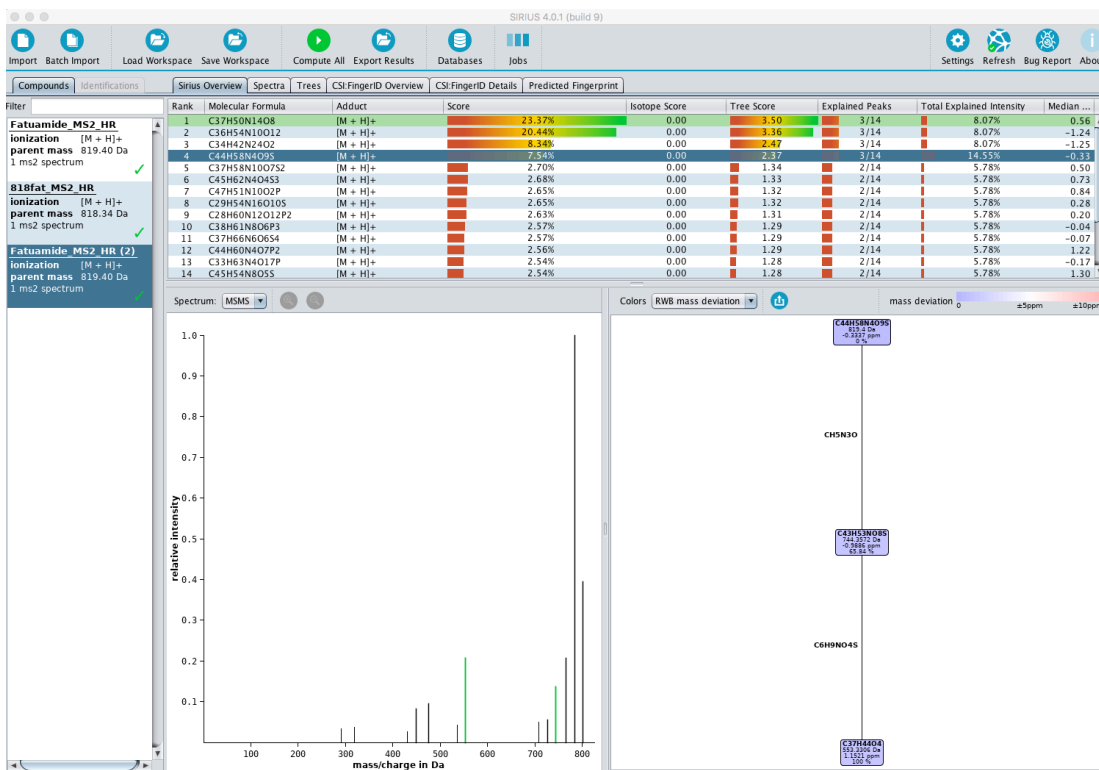
Figure 3.7: Analysis of the MS/MS spectrum of fatuamide A by SIRIUS 4.0 software. The blue highlighted formula was determined to be the molecular formula.
