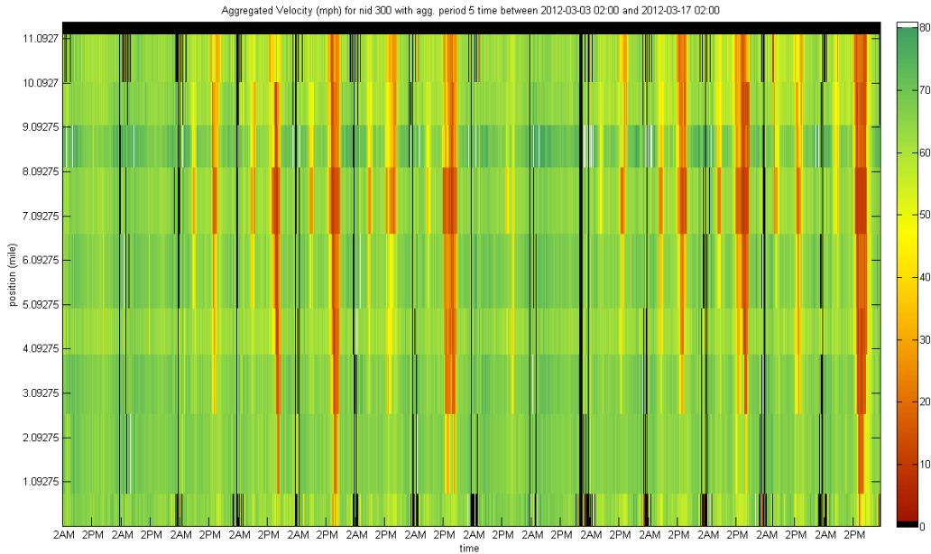
Figure 3-86: Bluetooth aggregated travel times (displayed here as velocities) for the “average time” strategy on I-880
