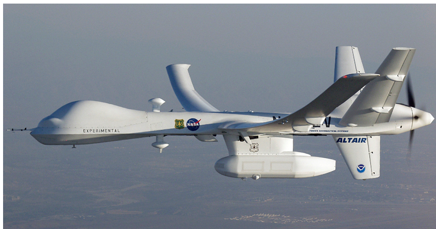
Figure 1.1: Altair Predator B, a UAV used by NASA for environmental research, http://www.dfrc.nasa.gov/Gallery/Photo/Altair_PredatorB/Medium/ED06-0208-1.jpg (webpage accessed on September 27, 2010).
