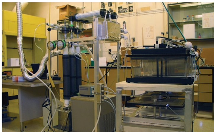
Rats were exposed to airborne particulate matter via an aerosol concentrator (VACES) in inhalation chambers.
