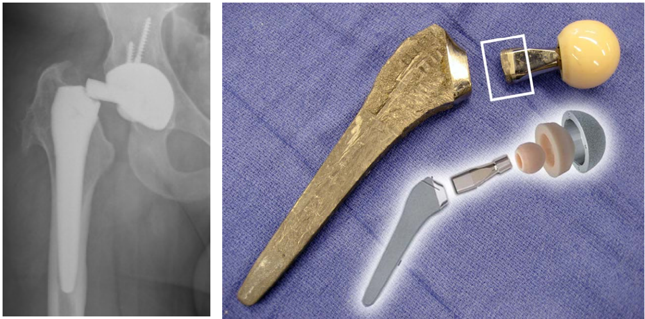
Figure A.2. (Left) Anterior-posterior radiograph showing fracture of the modular neck. (Right) The Profemur Z® retrieval with fracture of the modular neck component about 2 mm below the edge of the stem. The fractured region of interest (boxed) is shown in cross-section in Figure A.3 and in detailed side-view in Figure A.4.
