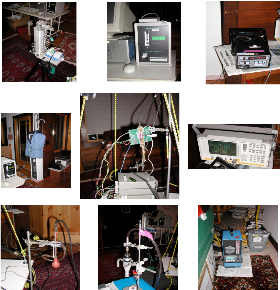
Figure 31. Field test instrumentation. Top row (L to R): Quartz crystal microbalance (QCM); aethalometer; optical particle counter (OPC). Middle row: High-flow sampler for measuring episodic source-enriched \text{PM}_{2.5} ; MEMS PM monitor; spectrum analyzer displaying FBAR resonance. Bottom row: Bubble flowmeter for use with MEMS PM monitor; FRM sampler for \text{PM}_{2.5} ; pump and gas meter for FRM sampler.
