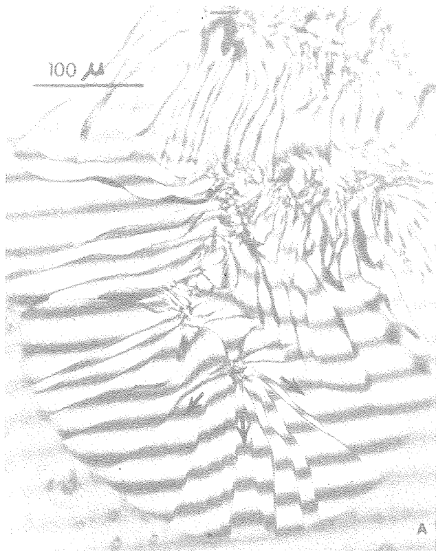
Fig. 2. Optical interferometry revealing the structure of a sodium filled cleavage crack induced by direct current passage through a single crystal of sodium beta alumina. (XBB 7811-14127)
