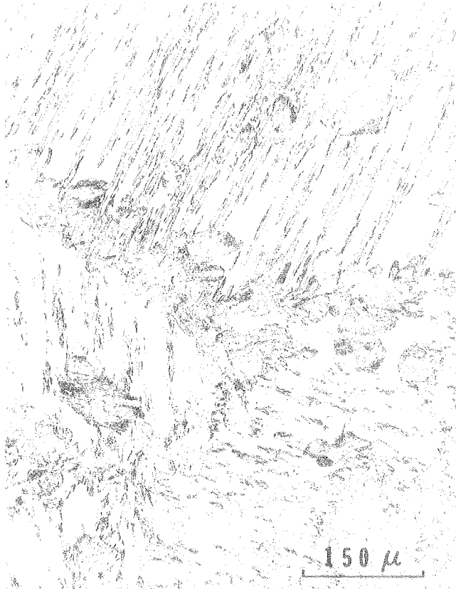
Fig. 1. Optical micrograph of DP structure developed in alloy 1 (Fe/0.5Cr/0.06C). (XBB 778-7550)
