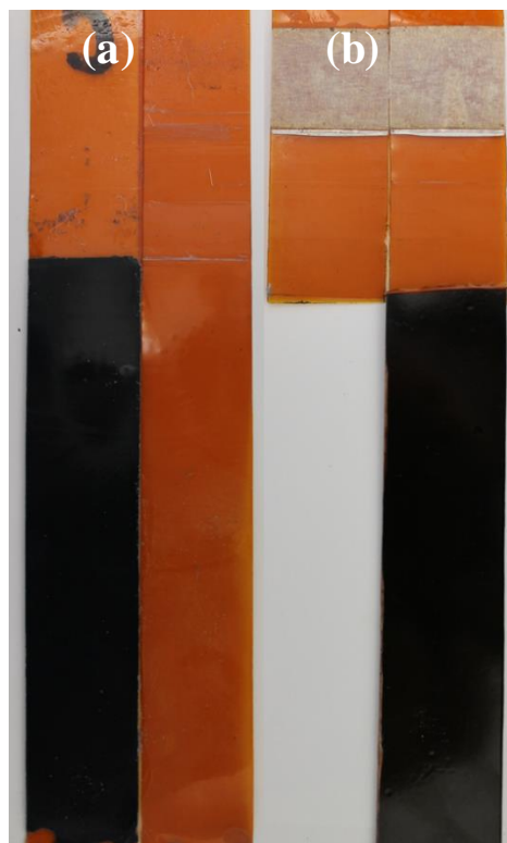
Figure 2.15. T-peel failure mode of polyimide (PI) samples is (a) interfacial for PI not treated by atmospheric pressure He/O 2 plasma treatment, and (b) cohesive in the polymer for PI treated by the plasma treatment.
