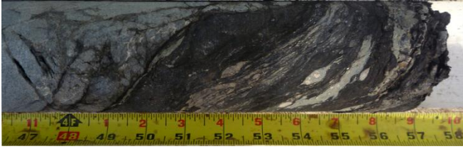
Figure 6 The core of foliated cataclasite at 92m depth in WF-2 consisting of highly sheared, anastomosed, stretched fragments of light yellow soft to hard siltstone and light gray sandstone embedded in a matrix of sheared black shale.
