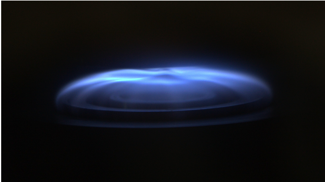
Figure 3.13: Photograph of an nonpremixed methane-air flame with a fuel mass fraction Y_{F,1} = 0.14 at 1.6 MPa displaying radial streaks.
