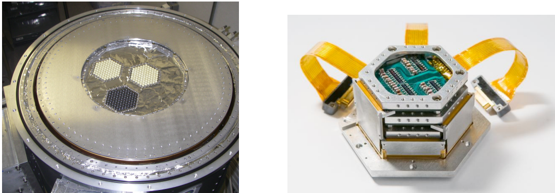
Figure 7.1: (a) Picture of the focal plane as it was deployed to Cedar Flat in early 2010. The white lenslets are alumina lenslets that were used for the early arrays because of their low cost. The darker lenslets are the observation-quality single-crystal silicon lenslets. All the lenslets are anti-reflection coated with thermoformed polyetherimide. For the Chilean deployment, the focal plane will consist of seven sub-arrays, all close-packed. (b) Picture of one of the sub-array modules, from the side that shows the frequency-domain multiplexed readout hardware. Note that the circuitry all fits behind the sub-array, to allow for close-packing of the sub-arrays in the actual experiment.
