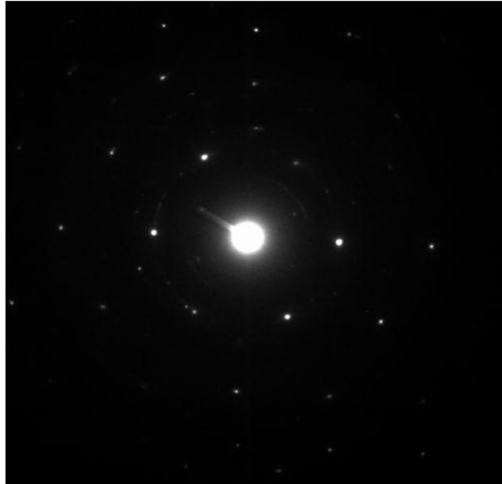
Figure 7.5: Electron diffraction pattern of individual exfoliated \text{Bi}_2\text{Te}_3 film indicating crystallinity of the films.
