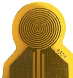
Figure 3.1: TPS nickel bifilar sensor with kapton insulation. Nano-Device Laboratory, UCR.
