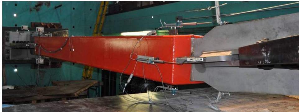
(a) Specimen 1 Overall, after Compression Proof Protocol
