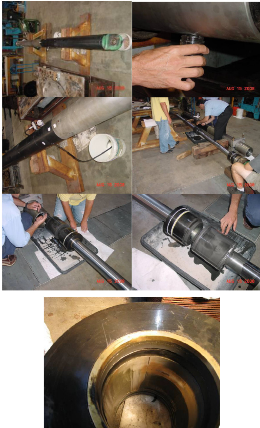
Figure 2.3 Photos of VTB Damper Disassembly and Internal Damage (Graziotti 2010)
