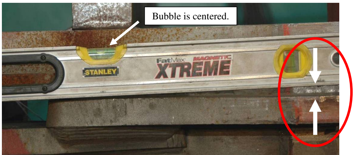
(b) Close Up, Brace Hinged within Core Plate
