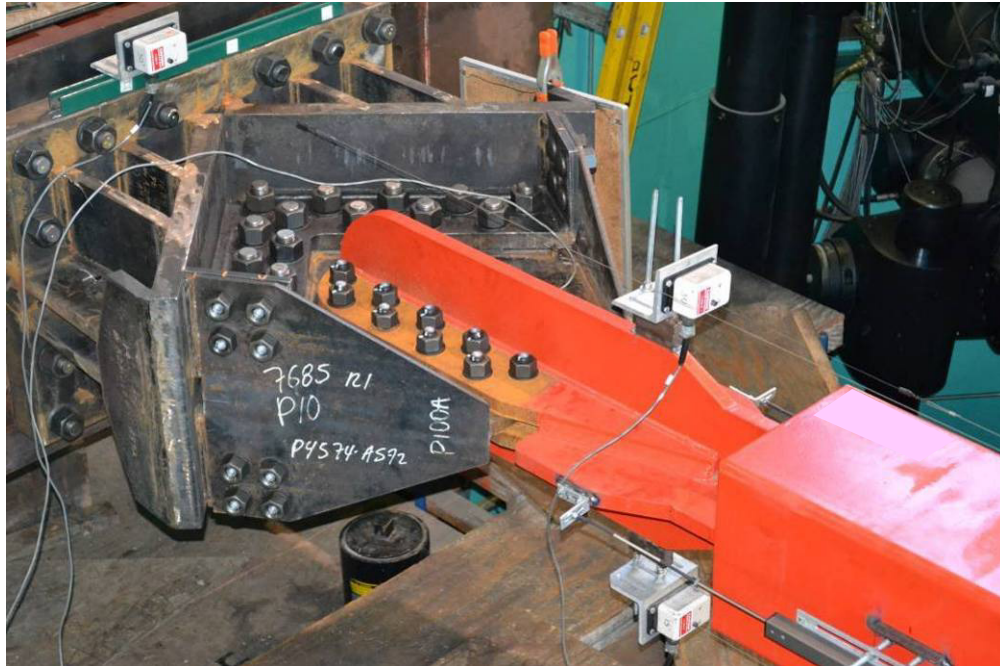
(a) Wall End Support (West End)
