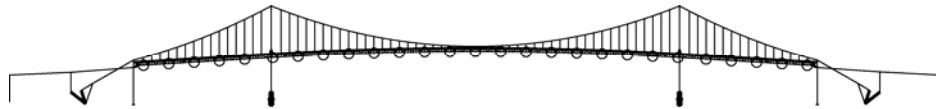
Figure 4.4. Locations of spatially discretized aerodynamic forces (“aerodynamic” nodes) along the bridge deck
