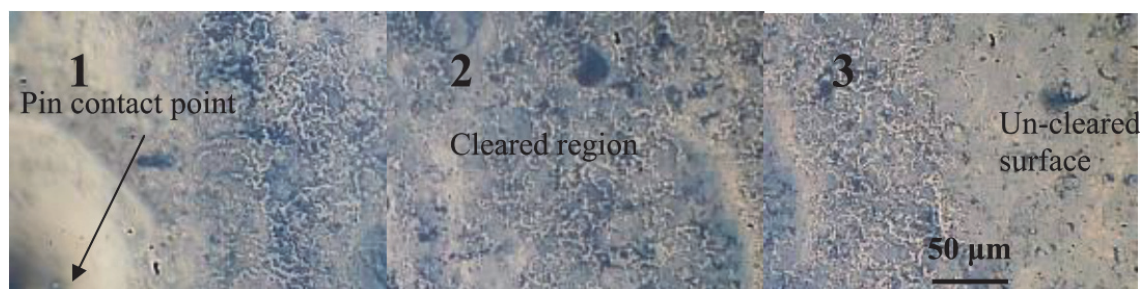
Figure 1.36 P3DOT:NOSbF 6 electrodes on a prestrained VHB™ actuator, magnified to the vicinity of the pin contact point and self-cleared region surrounding it. The de-doped, self-cleared region has a blue color, in contrast to the transparent un-cleared area. [114]
