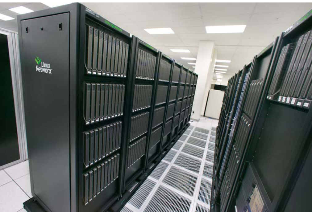
FIGURE 7. Jacquard is a 722-processor Linux Networkx Evolocivity cluster system with a theoretical peak performance of 2.8 teraflop/s.
