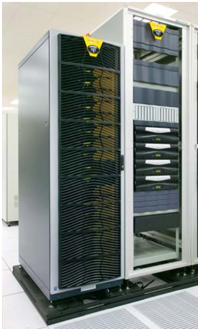
FIGURE 9. DaVinci is a 32-processor SGI Altix with 6 GB of memory per processor and 25 TB of disk memory, a configuration designed for data-intensive analysis and interactive visualization.
