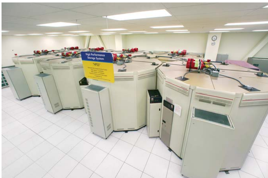
FIGURE 14. NERSC's High-Performance Storage System (HPSS) is capable of storing and retrieving all of JGI's genomic data efficiently.
