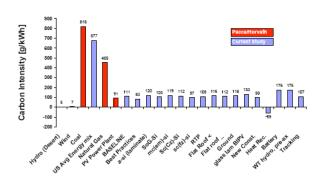
FIGURE 1. GLOBAL WARMING POTENTIAL [CO<sub>2</sub> EQUIVALENT] PER KWH, FOR DIFFERENT ENERGY PRODUCTION TECHNOLOGIES.
