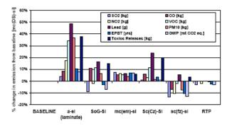
FIGURE 3. VARIOUS ENVIRONMENTAL METRICS ARE SHOWN COMPARING FEEDSTOCK OPTIONS, WAFER MATERIALS, AND PROCESSING CHOICES.
