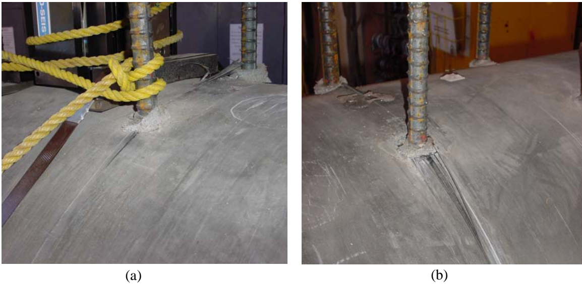
Fig. 5.24 Composite shell failure at location of stirrup holes: (a) near accelerometer a3, and (b) near accelerometer a7
