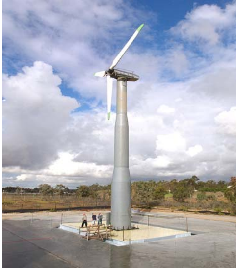
Figure 3.1: NEES-UCSD LHPOST with a full-scale 21m high wind turbine mounted on it.
