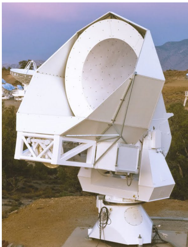
Figure A.2: The Huan Tran Telescope (HTT) at the James Ax Observatory deployed for an engineering run in Cedar Flat, California. The secondary mirror and receiver (not installed here) are positioned inside the truss structure below the primary mirror. Part of the CARMA telescope array is visible in the background.
