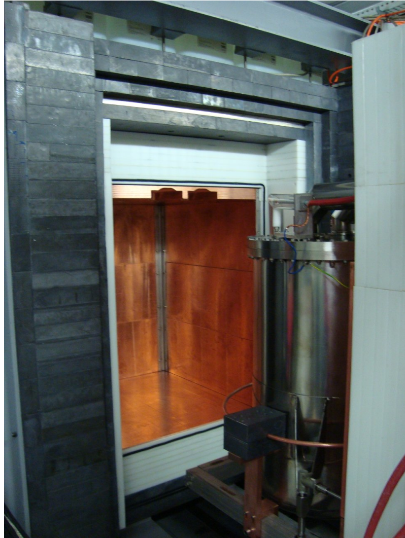
Figure 2.6: External shielding enclosure and cryostat attached to the right wall. The shield is composed of two layers of lead, polyethylene, and copper. The stainless steel cryostat has a copper ring surrounding it for detector calibrations.
