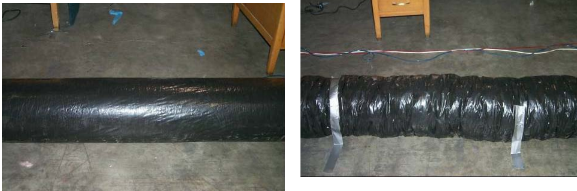
Figure 3 The exterior of the fully stretched, and the compressed (29.50%) 10” (250 mm) flexible duct test specimens.
