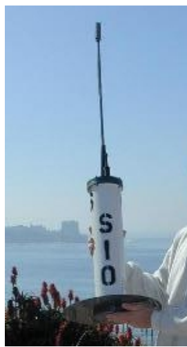
Figure 1: Schematic of the surfzone drifter. Surface piercing antennae for receiving GPS signals and for radio-frequency (RF) communication with shore are molded permanently to the drifter top cap. A 6-pin port, also integral to the top cap, permits programming and data downloading (I/O), and battery charging without opening the drifter package.
