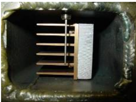
Figure 3 - Installed Thermocouple Probe and Electrical Heater Block 2.0 in wide by 6.0 in long
