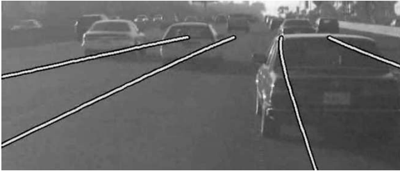
Fig. 16. Error due to occlusion of the road by a vehicle on the dusk dataset on road segment C.
