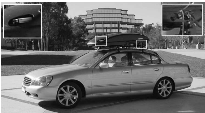
Fig. 10. LISA-Q intelligent-vehicle test bed. Inset are close-up views of the front camera (left inset) used for detection and tracking and side camera (right inset) used for generating ground truth.
