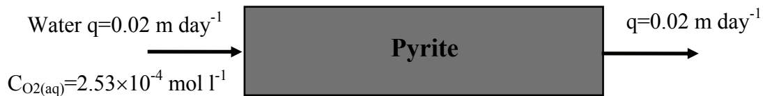
Figure 2. Schematic representation of the 1-D horizontal saturated flow system used for pyrite oxidation.
