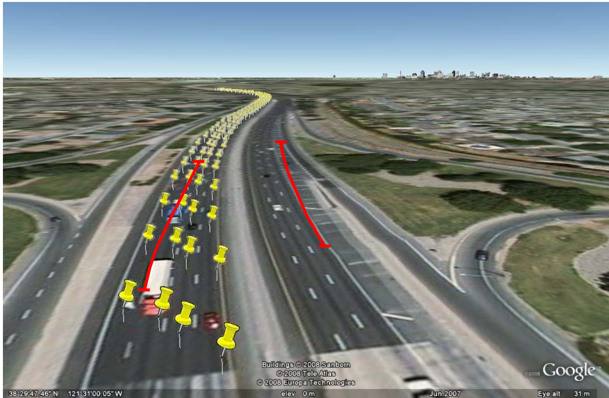
Figure A.19: Depiction of southbound lanes tested over the whole length and the approximate location of monitoring sections (red lines) in the northbound and southbound outer lanes.
