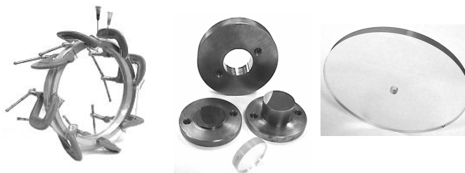
Fig. 4. Polymerization cell, compression mold and fabricated WORM disk.
