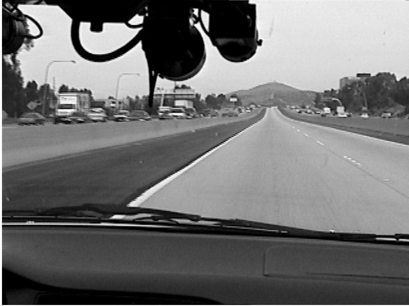
Figure 5: View from inside the automated Honda accord showing the mounting of the cameras
