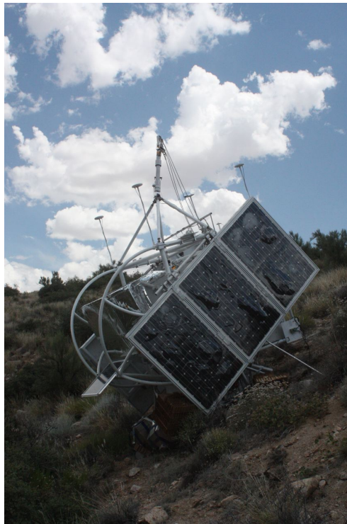
Figure 7.3: The gondola on the ground after the termination of the flight. Note that the gondola landed upright, which allowed the liquid nitrogen to remain in the dewar so the detectors remained at cryogenic temperatures. Also apparent is the bubbling and cracking damage sustained by the solar panels during flight.
