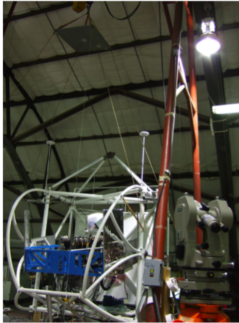
Figure 3.11: Setup for the effective area calibration. The theodolite used for placement can be seen in the lower right corner, and the board used for source placement and sighting can be seen in the upper left. The sources were placed 5 m away from the detectors.
