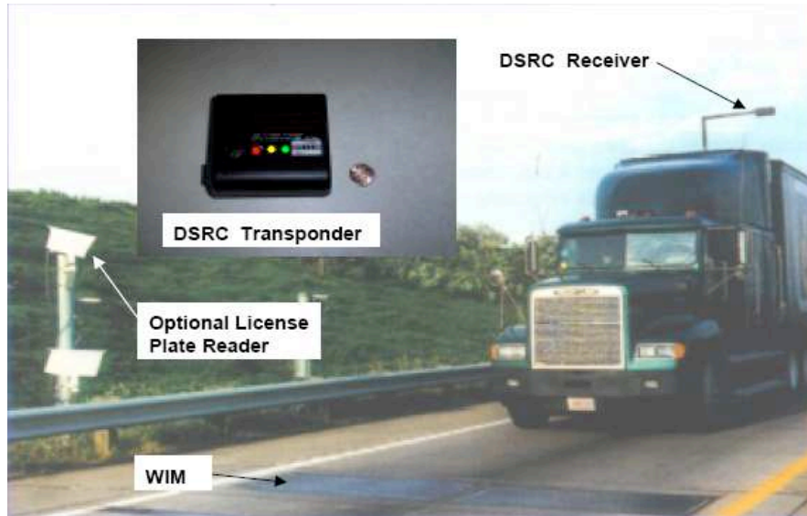
Figure 7. Electronic Screening Using DSRC Technology
