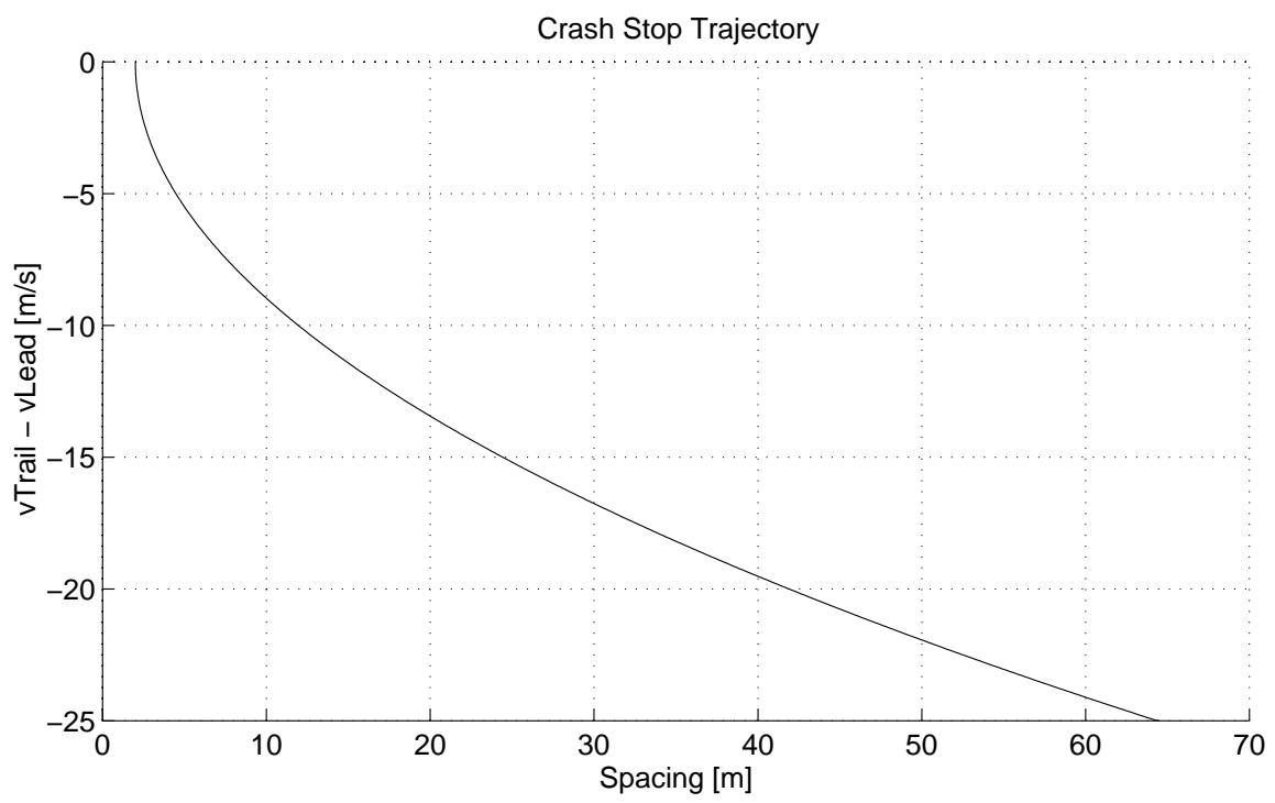
Figure 12 Crash Stop Maneuver Safety Boundaries and Performance
