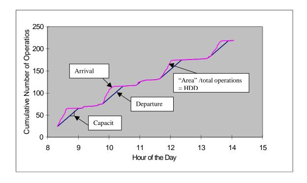
Figure 2: Method for Computing Hypothetical Deterministic Delay (HDD)
