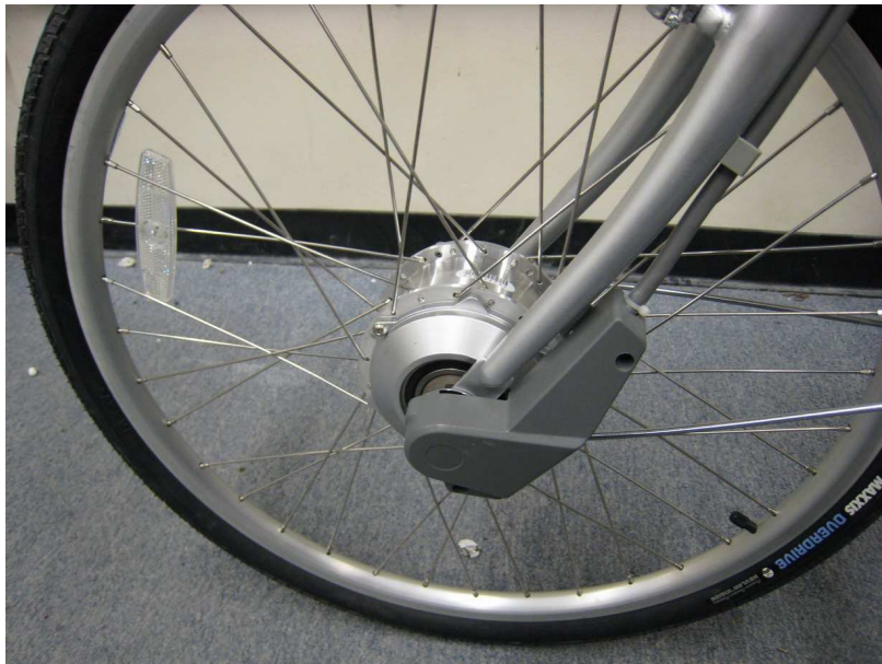
Figure 2.4: Electric hub motor in the front wheel
