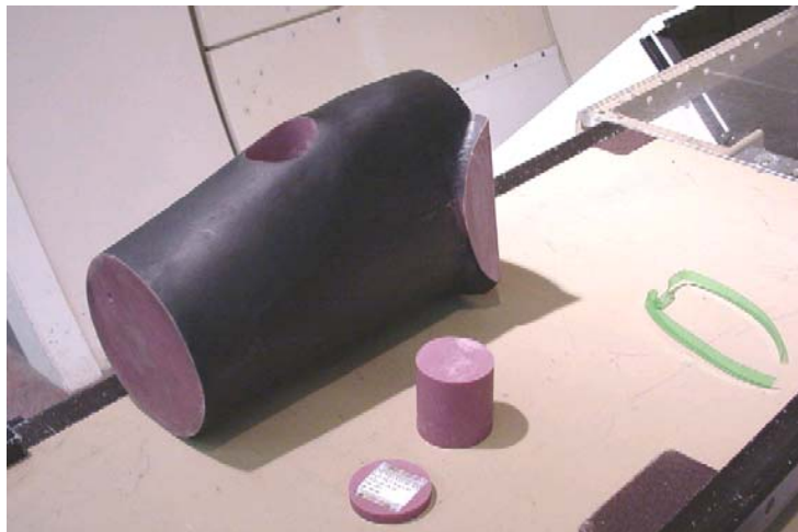
Figure 11. A part of the phantom's right thigh, detector stack, and tissue equivalent plug used in making irradiations of the thigh location while inside the EMU suit.
