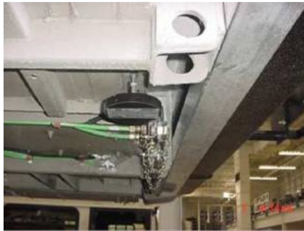
Figure 4-21: Inductive Loop Transponder Mounted on Underside of a Bus
