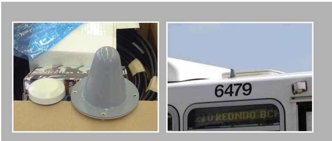
Figure 4-10: Typical GPS and Wireless Communications Antenna Installation
