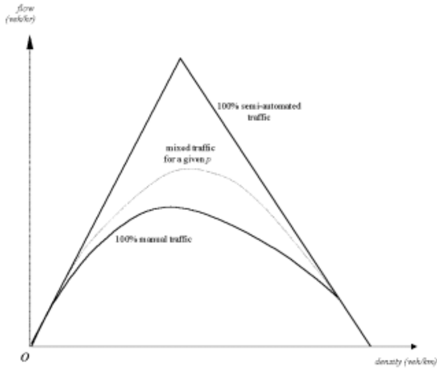
Figure 7: Fundamental q - k diagrams for 100% semi-automated, 100% manual and p mixed traffic at steady state conditions.
