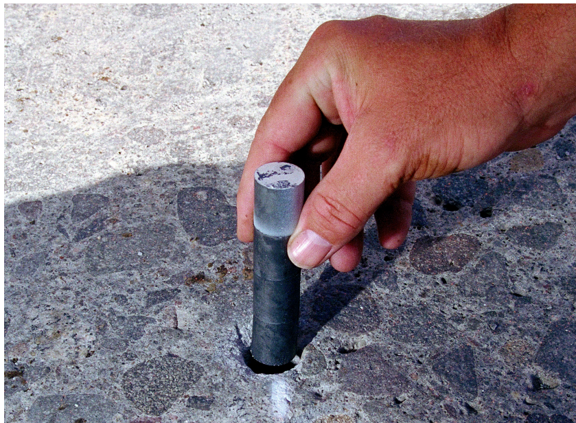
Figure 1. An exemplar marker before insertion into a hole in the roadway pavement
