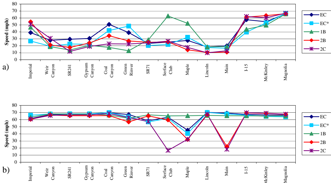
Figure 4.8. Speed trace for the eastbound pm SR-91 by scenario for per mile rate level1 for a) general purpose lanes and b) HOT lanes.
