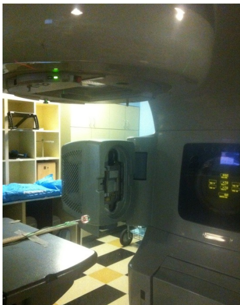
Figure 3.7: Isocentric setup to obtain the diode symmetry property.
