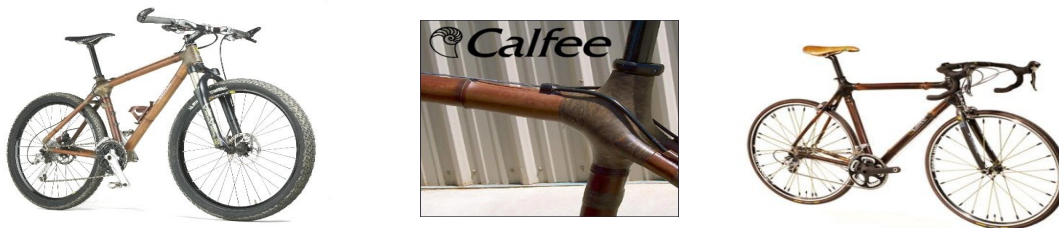
Illustration 49: Calfee designs high-performance bamboo and hemp composite bikes.
